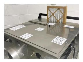
• **Inspect filters** regularly and replace if dirty. Regular air filter maintenance is critical to extending the life of the desiccant rotor and moisture removal efficiency.
